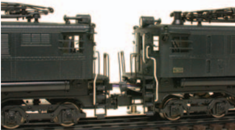
On 3-rail O-1s, the control unit has coil couplers while thumbtack couplers are on the booster unit.
