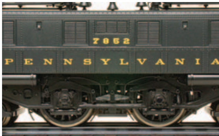
Driver axles run in sprung journals. Although the equalizers move, they are non-functional.
