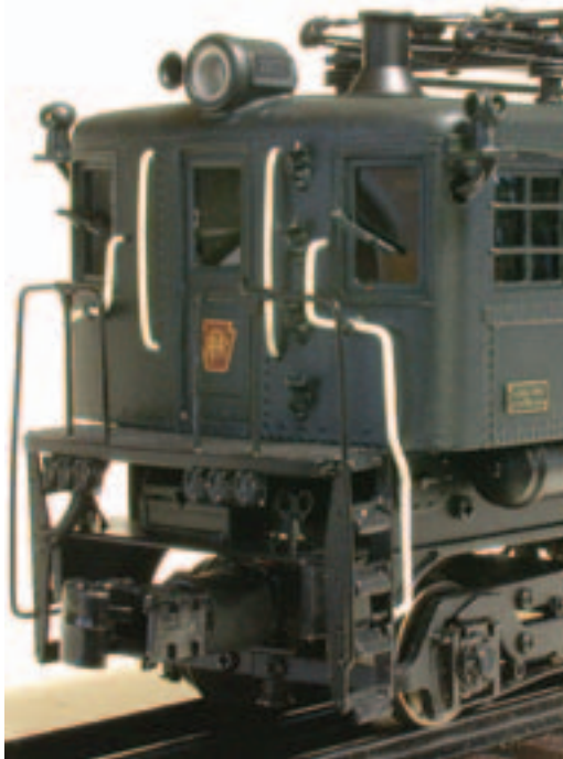
Casting representing the MU cable receptacles are visible below the walkway. The large tinplate coupler inhibits installation of a pilot.
