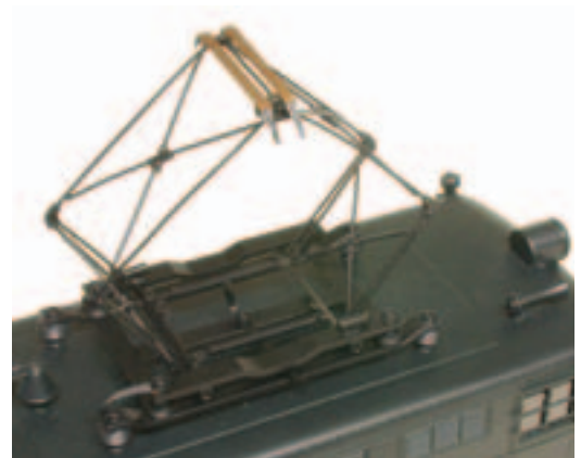
A manually operated retaining lever releases the operating and functional pantograph to the raised position.
